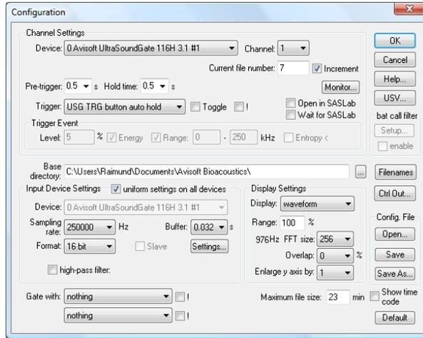
The input sample rate can be selected from the **Input Device Settings** section. Available sample rates are 750, 500, 375, 300, 250, 214, 187, 166, 150, 125, 100, 75, 62 and 50 kHz.
